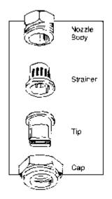
**Nozzle tips** break the liquid pesticide into droplets. They also distribute the spray in a predetermined pattern and are the principal element that controls the rate of application. Nozzle performance depends on: nozzle design or type, operating pressure, size of the opening, discharge angle, distance of nozzle from the target.
